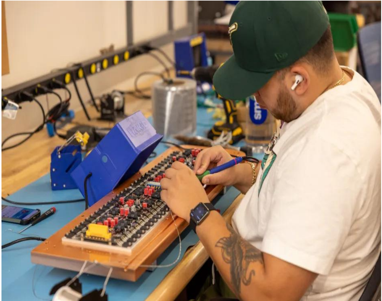
Relentless Epic 1600 output stage being carefully constructed.
